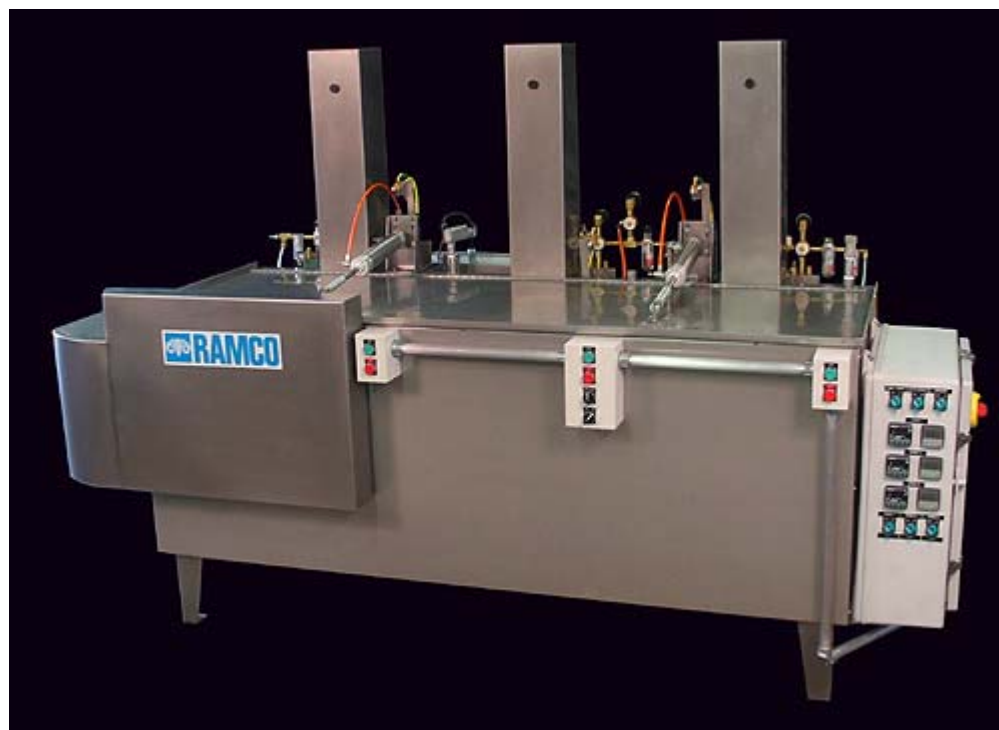
This application is a Passivation System for medical components. The standard MKT24WRR is constructed from type 316L stainless steel. The process uses heated nitric acid. The line runs left to right.
